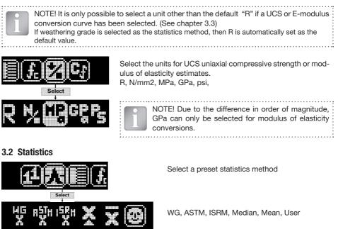
The WG (weathering grade) method requires two impacts to be carried out on exactly the same test location. The difference between the two impact values is calculated and displayed. Please refer to the ISRM guideline for a complete explanation.
